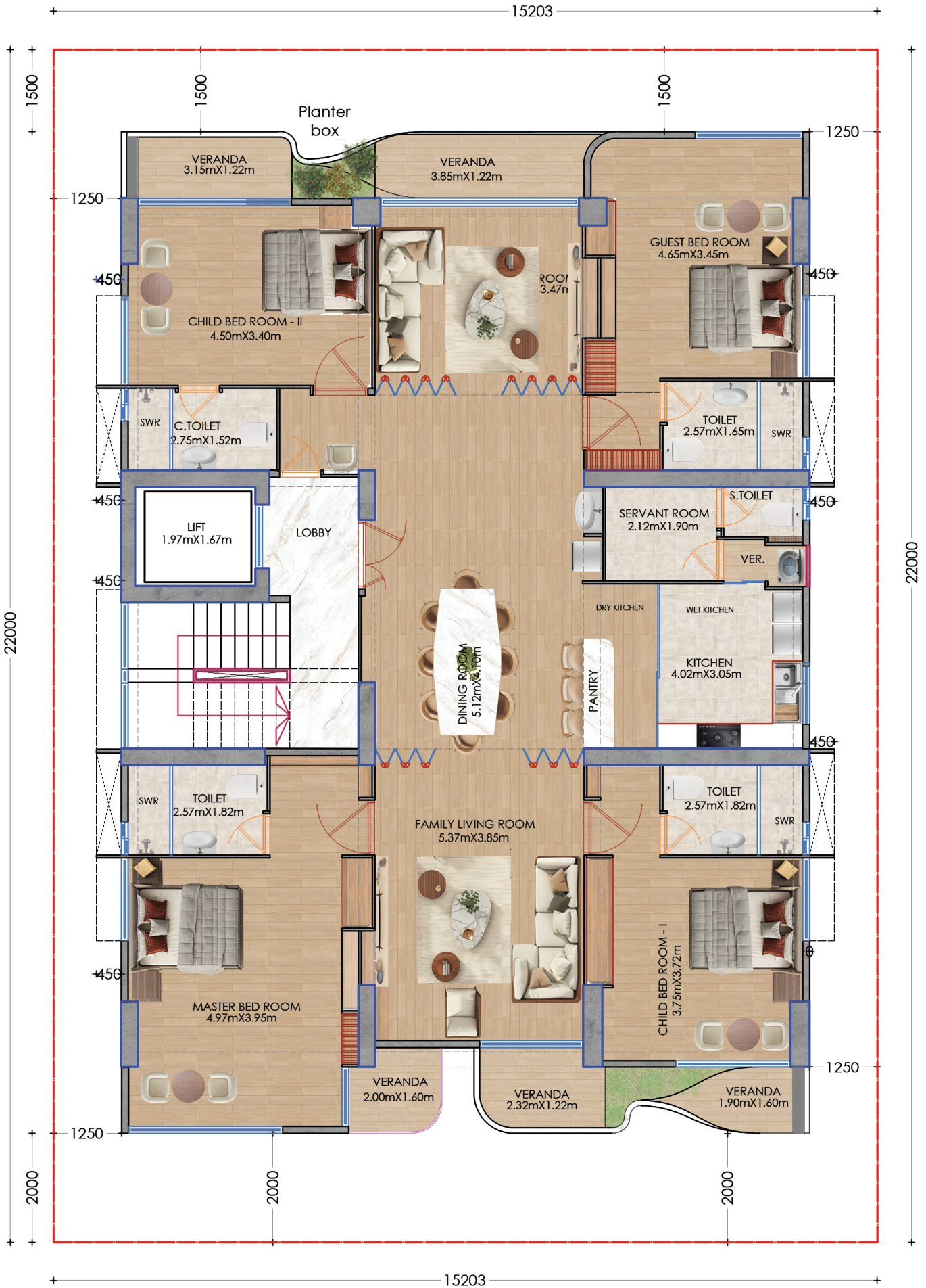
2nd, 4th, 6th & 8th FLOOR PLAN Scale- 1:100
